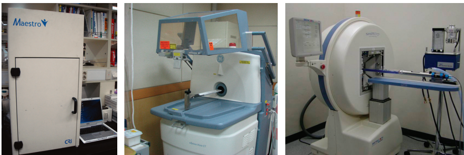
새롭게 설치된 분자영상장비들, 광학영상장비, 소동물 PET/CT, 소동물 SPECT/CT Newly installed molecular imaging facilities
